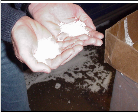
Figure 3 Beads of PS and EPS
