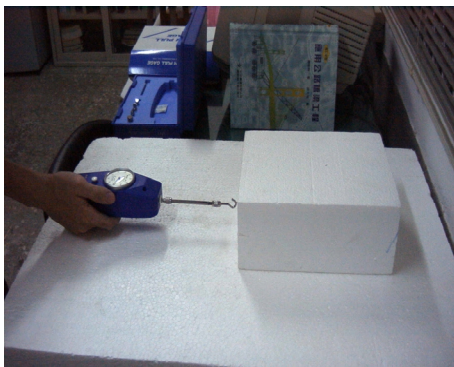
Figure 14 EPS friction coefficient test
