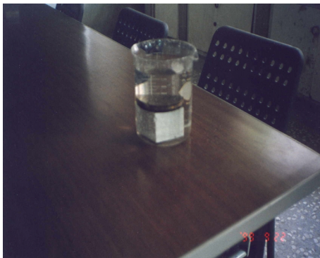
Figure 12 EPS sample in moisture absorption test
