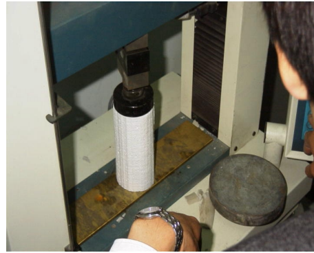
Figure 17 EPS single axis test
