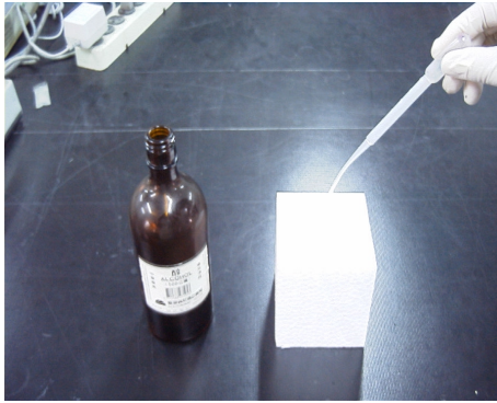
Figure 16 EPS surface erosion test
